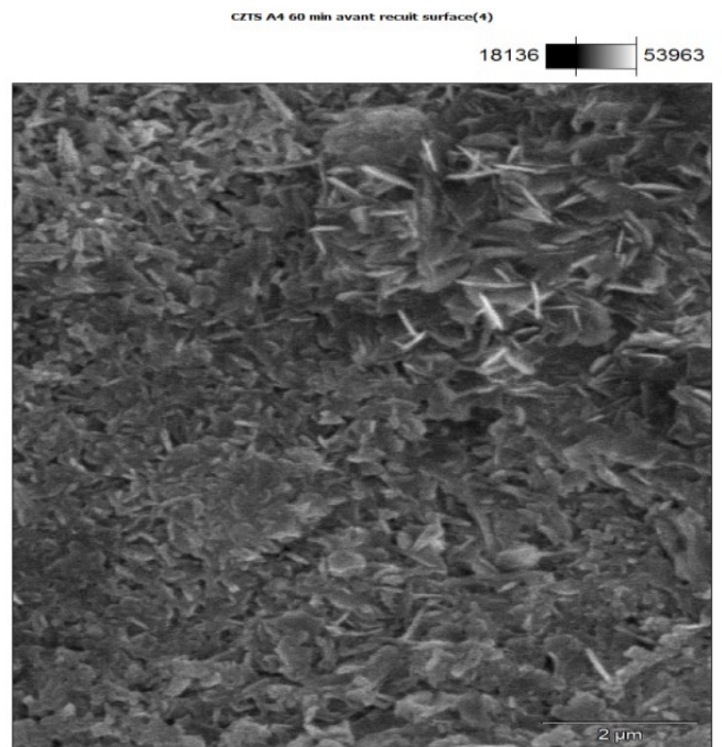
Fig. 5: SEM micrograph of CZTS samples deposited at 60min duration spray before annealing
